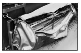
2. With the tonneau cover rolled up, place it in the proper compartment in the bag and zip the bag shut.
